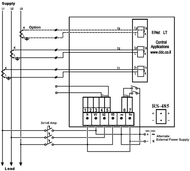
Figure 2.4 Schematic Wiring Diagram "Delta" connection
